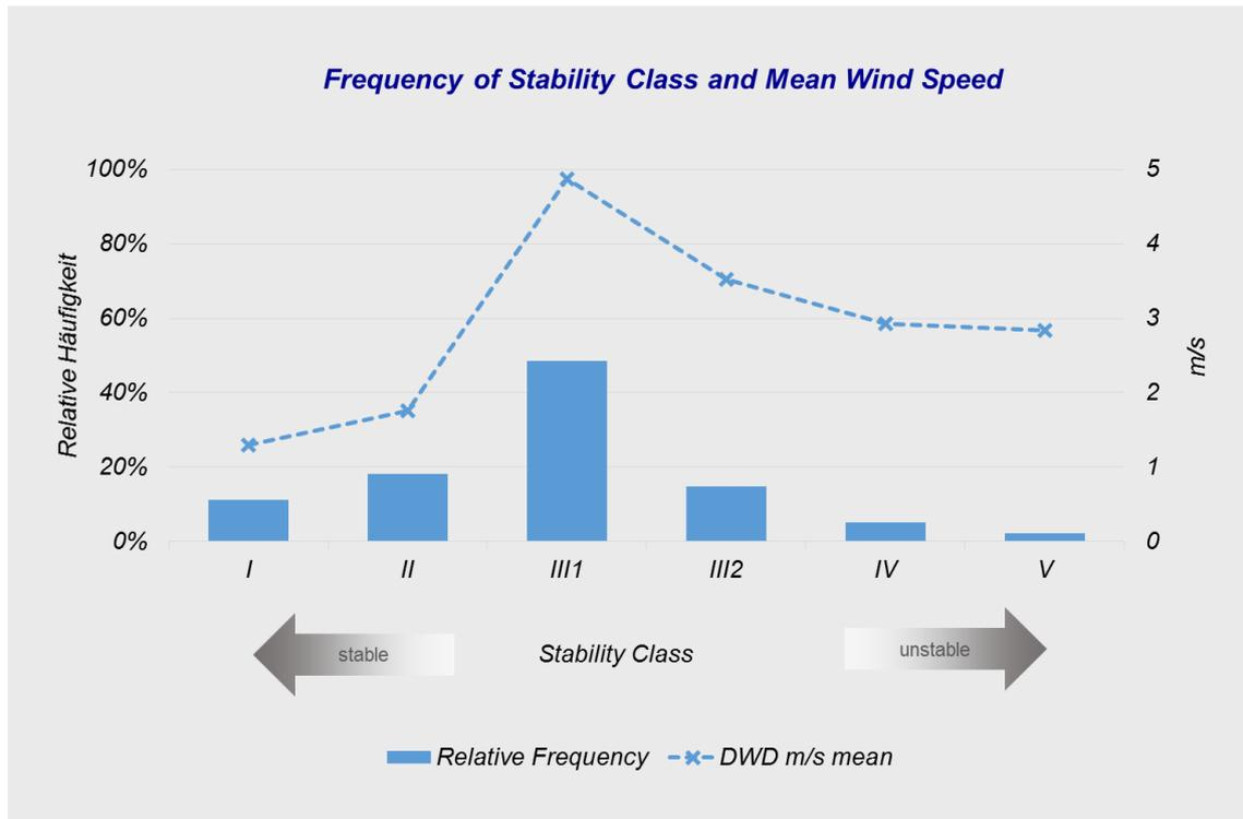
Evaluation of hourly data WebWerdis according to VDI 3782 (2009)
