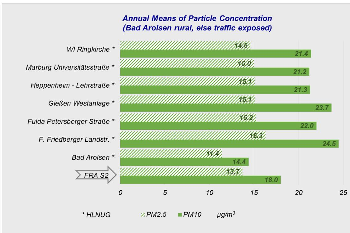
The average PM2.5 to PM10 ratio slightly depends on the location and is between 60% and 80% at all sites. At the airport, it amounts to 76%. Insofar, PM2.5 monitoring has not lead to basic new discoveries. With respect to air quality surveillance, PM10 continues to be a substantial measure, not least because a short-term limit exists, which however has not been exceeded in Hesse after 2011.
